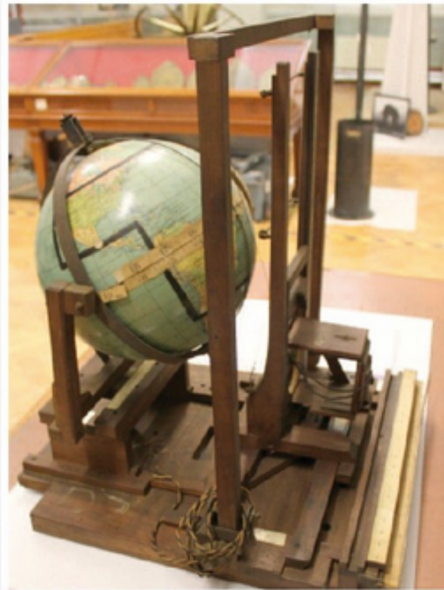
Figure 2. McNeille's wooden Occultation Machine. (Science Museum/Science & Society Picture Library)
